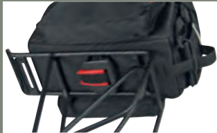
Push forward to fix the bag
